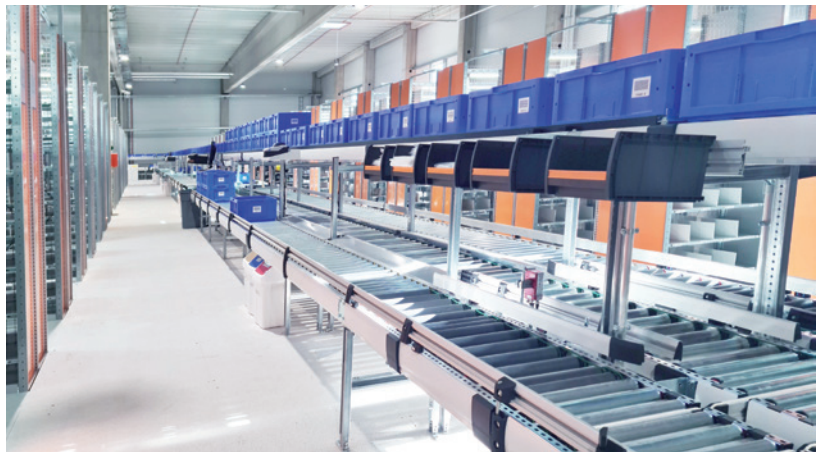
Shelving system with conveyor technology
