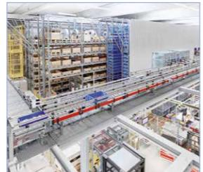
Göpfert – automated container, pallet and shuttle warehouse with production connection
