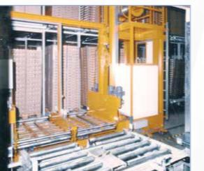
Pallet storage and retrieval system in operation at Gervais-Danone
