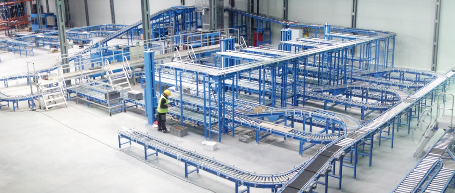
The shuttle warehouse is connected via conveyor technology to 6 order picking and 16 shipping stations
