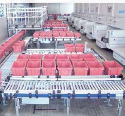
18 lift storage areas with 9 order picking stations and automatic replenishment buffer
