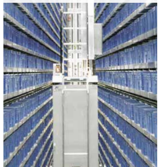
3-aisle automatic tray warehouse
