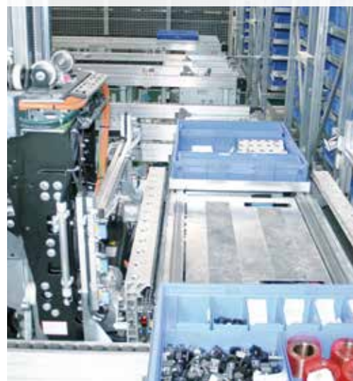
Automatic storage and retrieval crane with drawing technology
