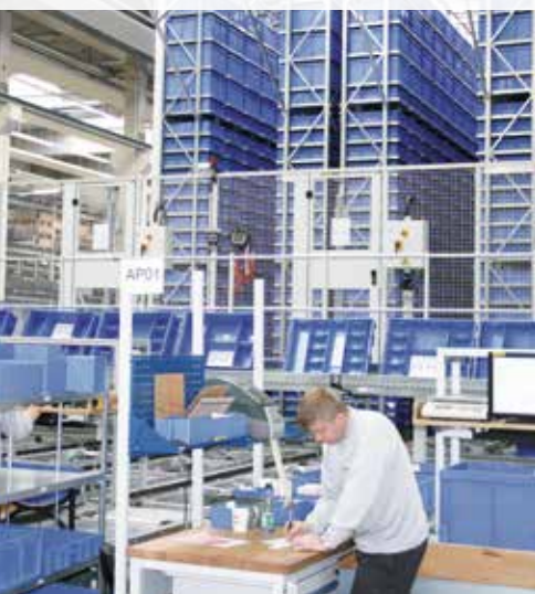
Order picking zone with 4 work stations
