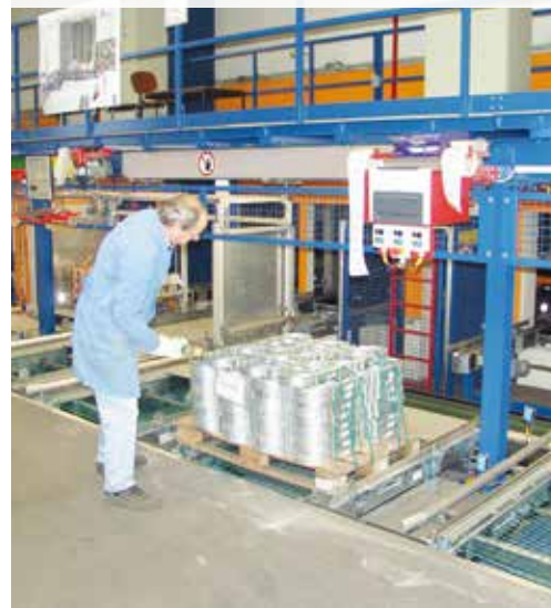
Picking zone: Three working places with three supply units each.
