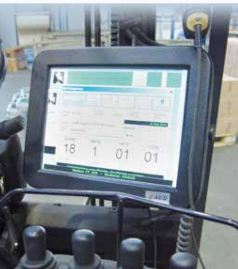
Stacker terminal: even in mobile mode fully LVS functionality
