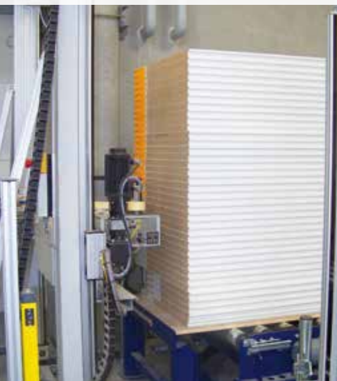
Automatic door scanning and labelling
