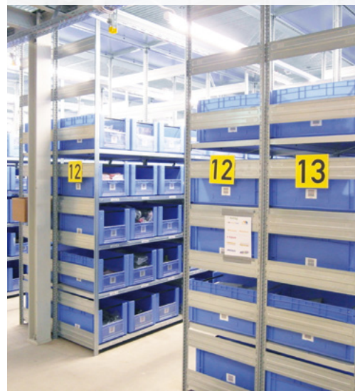
Shelf storage system with 21,000 container storage locations
