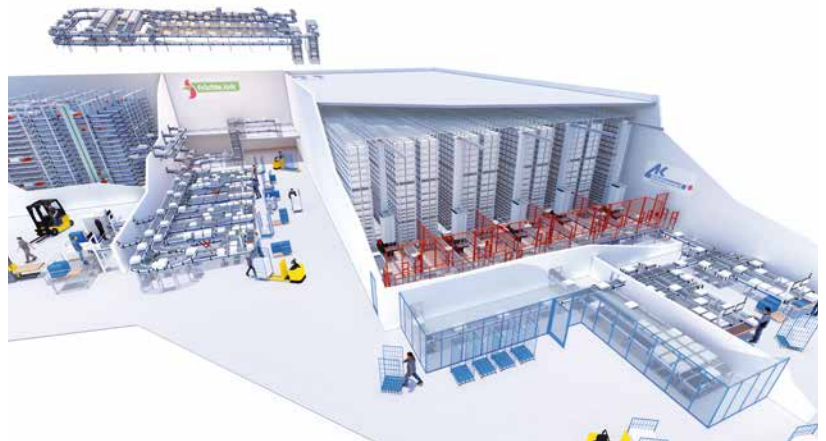
Logistics centre with shuttle warehouse and automated deep-freeze warehouse
