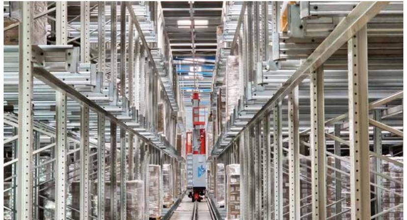
Single-aisle channel storage system for 2,100 pallet spaces
