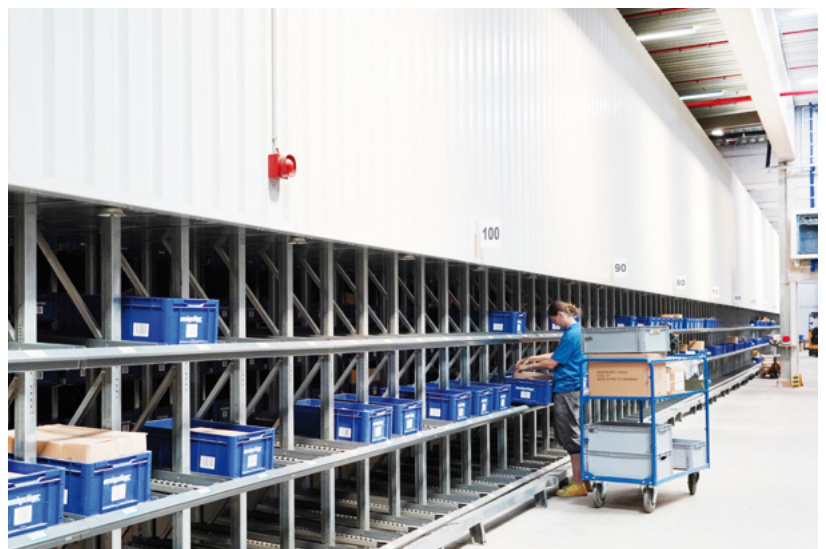
Retrofit of the 1-aisle, automated small-parts warehouse with lateral flow channels
