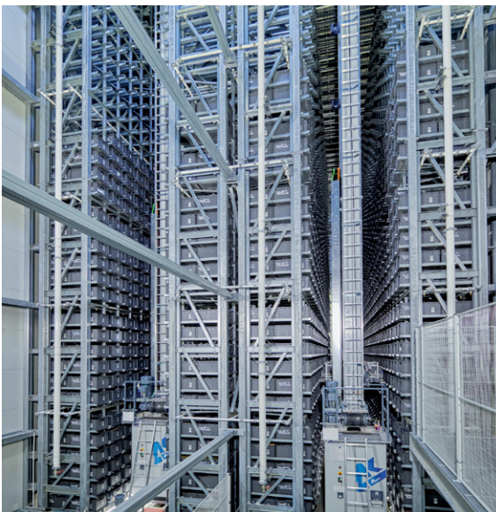
Automated small-parts warehouse for 8,120 bins
