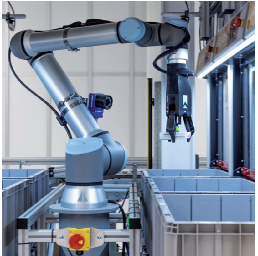
Fully automated robots pick from 6 bins into the target carton
