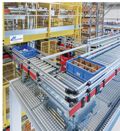
Pre-zone of the multilevel shuttle with conveyor-bridge
