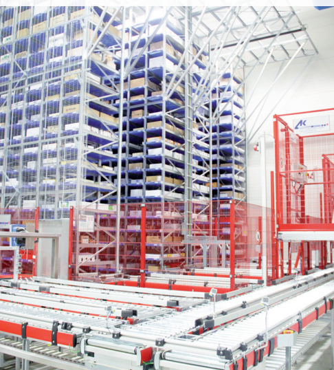
Deep-freeze warehouse with 19,680 tray storage locations
